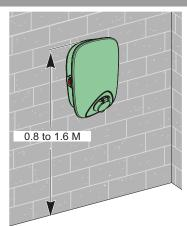
■ Check the installation area before marking it on the wall. It is recommended to situate the top of the charging station between 0.8 to 1.6 m above the ground.
