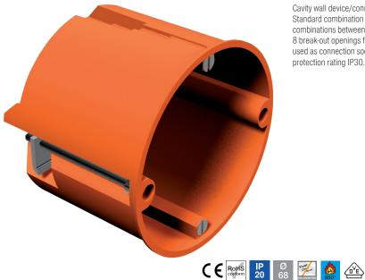
Cavity wall device/connection socket. Dimensions to DIN 49073-1, for plate thickness 7–35 mm. Standard combination spacing 71 mm, option for continuous wiring using connection support for combinations between device sockets and device connection sockets,
